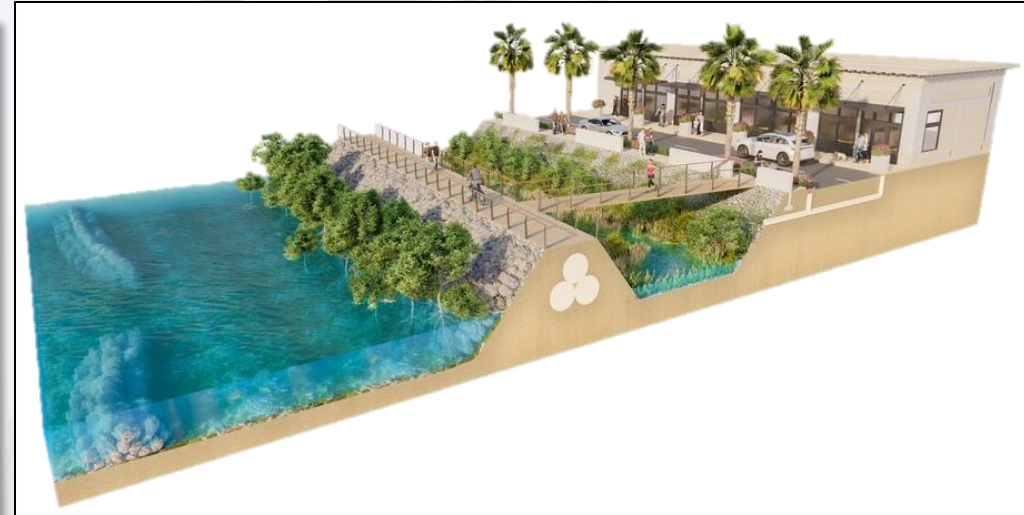
Above & Below: Renderings showing NBSs used in combination with wall/levee features.
