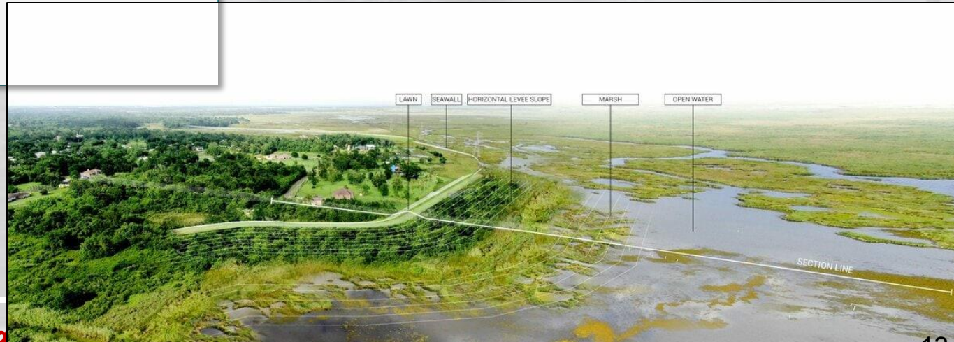
Above & Below: Renderings showing NBSs used in combination with wall/levee features.
